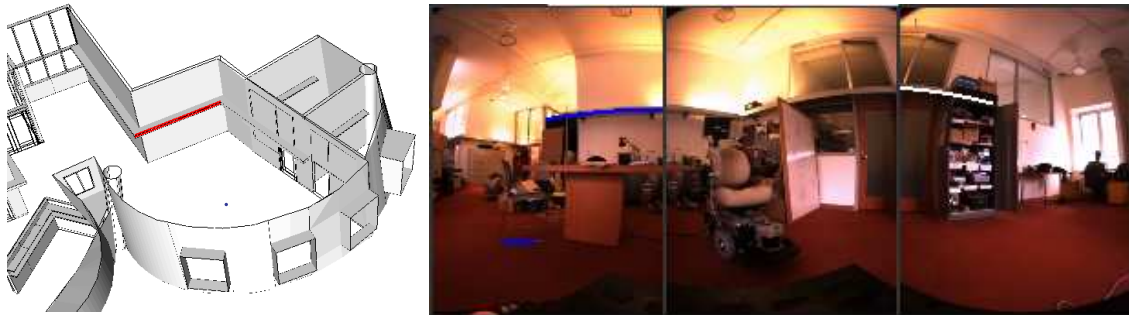
Figure 8-3: An example output of the fitness-based line matching algorithm. A 3D model line is selected on the left. The three best image edge matches for this line are displayed on the right. The system found the correct match (in blue on the left-most tile).
