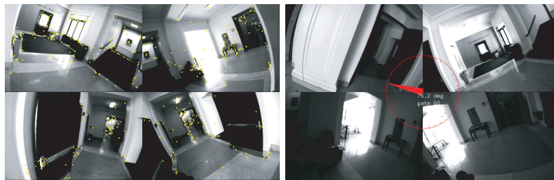
Figure 4-20: Left : first visit of a node (CORRIDORS dataset). Feature points are shown in yellow. Right : coming back to the same location during a homing scenario. The red compass shows the direction given to the user.
