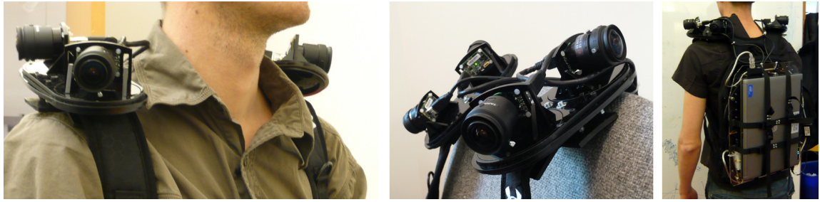
Figure 1-6: Our body-worn sensor suite includes four IEEE 1394 cameras mounted on the shoulders of the user, with a 360^\circ field of view.
