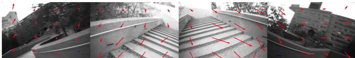
Figure 4-26: A frame classified as “ascent” as the user is walking up a stairwell outside the MIT Stata Center. Even though the environment looks different from the training setting (Figure 4-10), the classifier determines the motion category correctly.
