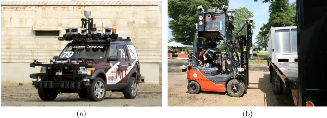
Figure 2-1: Both these autonomous vehicles require extrinsic sensor calibration to fuse data from multiple sensors.
