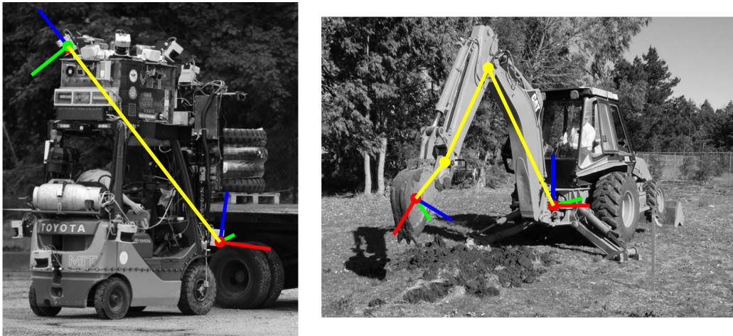
Figure 1-1: The sensors on a robotic platform (left) form a simple, rigid mechanical chain. The arm of a backhoe (right) forms a more complex mechanical chain with several joints.
