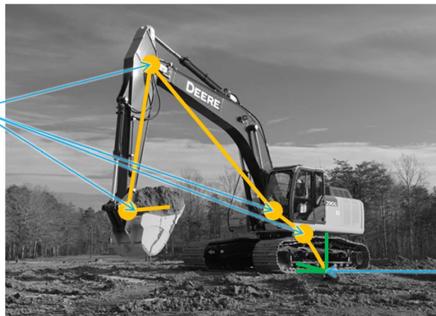
Figure 3-4: The goal of the articulated object tracker is to estimate the joint values and base pose of an articulated object, such as the excavator shown here. Observations might be image detections.
