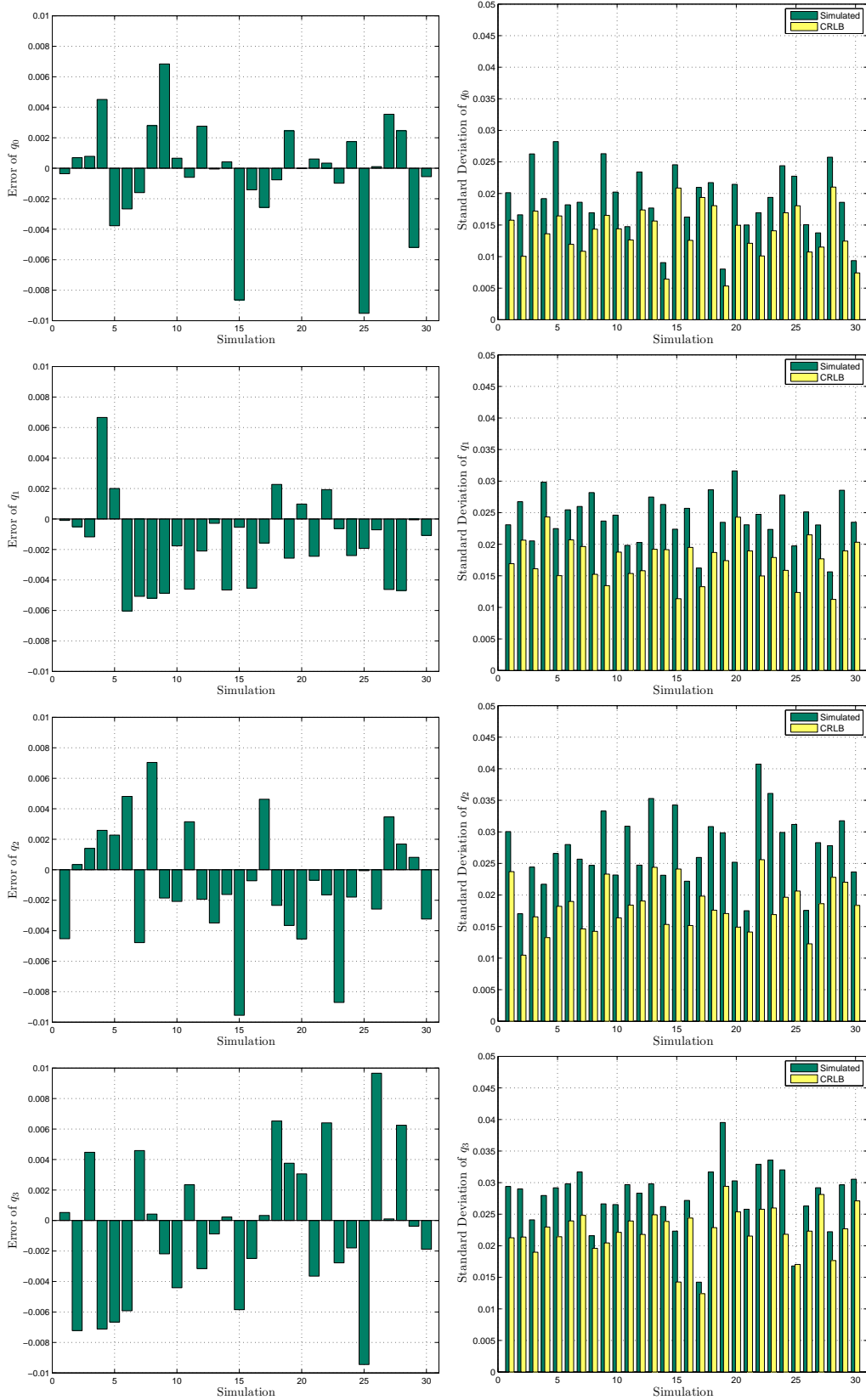
Figure 2-27: The error between the known calibration and the mean estimate was less than \pm 0.01 for each DQ parameter. Parameter q_0 - q_4 are shown here.
