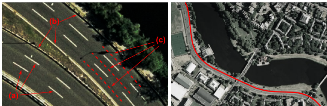
Figure 4-1: Left: Curves of interest in the context of lane estimation include painted lane boundaries (a), raised curbs (b), and (typically invisible) lane centerlines (c). Right: The spatial extent of curves can be much larger than a vehicle’s sensor range; in many cases estimates of the entire curve are not necessary.
