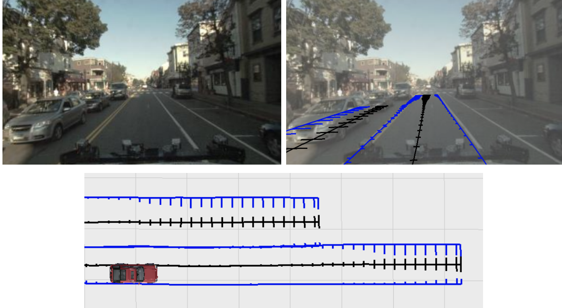
Figure 5-3: (top left) The farthest boundary of the opposite lane is occluded by other vehicles. However, by maintaining a joint distribution over centerline geometry and lane width, (top right) the system can still maintain an estimate of the opposite lane, using observations of the closer boundary. (bottom) A synthesized overhead view of the vehicle and its lane estimates. Black curves correspond to the estimated lane centerlines, and blue curves denote the marginal distributions of the lane boundaries. Short line segments extending laterally from the curves indicate control point uncertainty.
