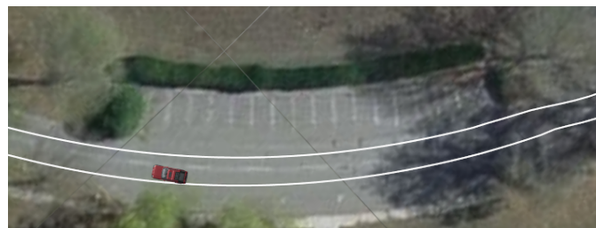
(c) Filtered and tracked lane centerlines
