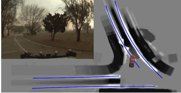
Figure 3-2: Lane centerline candidates (blue) are identified by fitting parabolic segments to the ridges of the evidence image (white). Front-center camera view is shown in top left for context.
