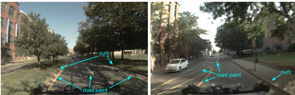
Figure 1-3: Feature detectors process sensor data to extract information useful for lane detection. The features considered in this thesis are painted markings and physical curbs. Other useful features may also include vehicles, traffic signs, and traffic lights.
