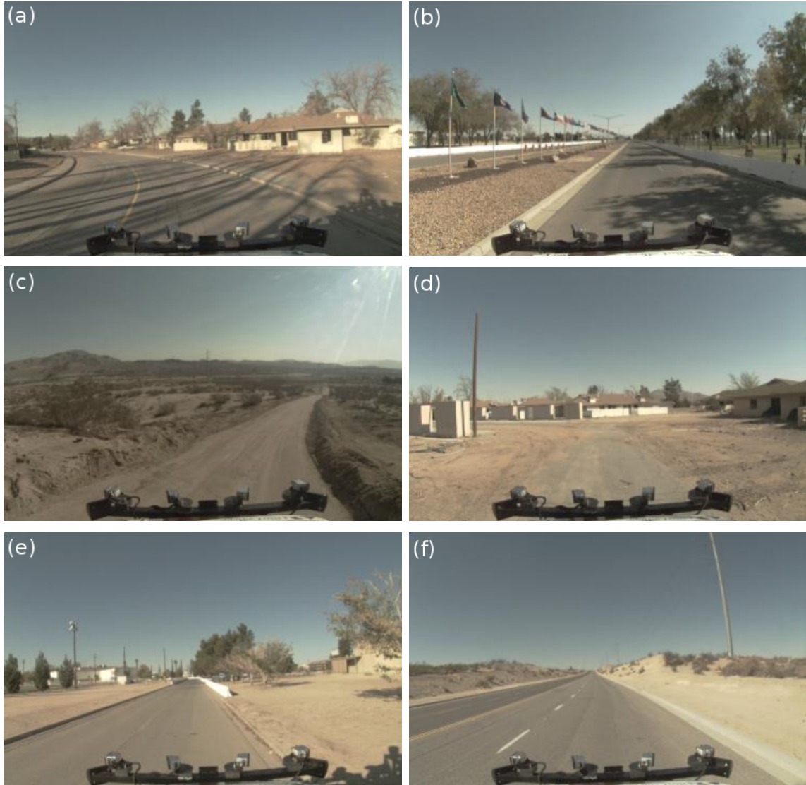
Figure 3-5: Common failure cases (cf. Fig. 3-4). The most common failure was in areas with strong tree shadows, as in (a) and (b). Dirt roads, and those with faint or no road paint (c-e) were also common causes of failure. In (f), a very wide lane and widely-spaced dashed markings were a challenge due to our strong prior on lane width. In each of these failure situations, the system reported no confidence in its visual estimates.
