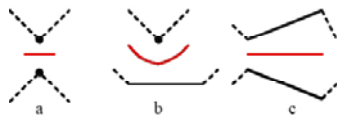
Fig.1-10: Shape of medial axis segments. (a) straight line between a concave-vertex pair; (b) parabolic arc between concave vertex and boundary edge; (c) straight line between two boundary edges [Joan-Arinyo 1996].
