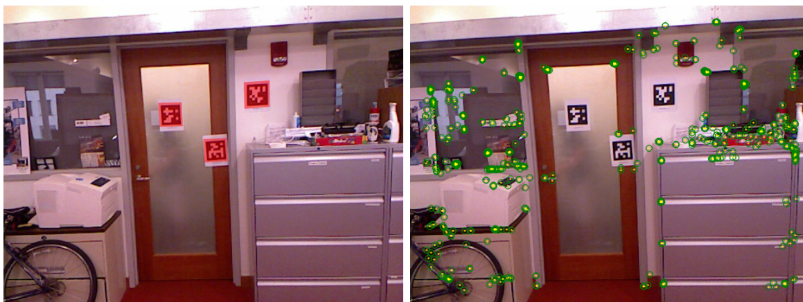
Figure 4-8: An example of the in-painted mask (in red) obtained via AprilTag detection, and the corresponding features extracted in the scene using the mask.
