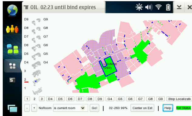
Figure 2-5: Spatial uncertainty. The user is shown their location estimate with a solid blue line around the room. The UI conveys the uncertainty of the estimate by stippling spaces that belong to the Voronoi region of the currently estimated room.
