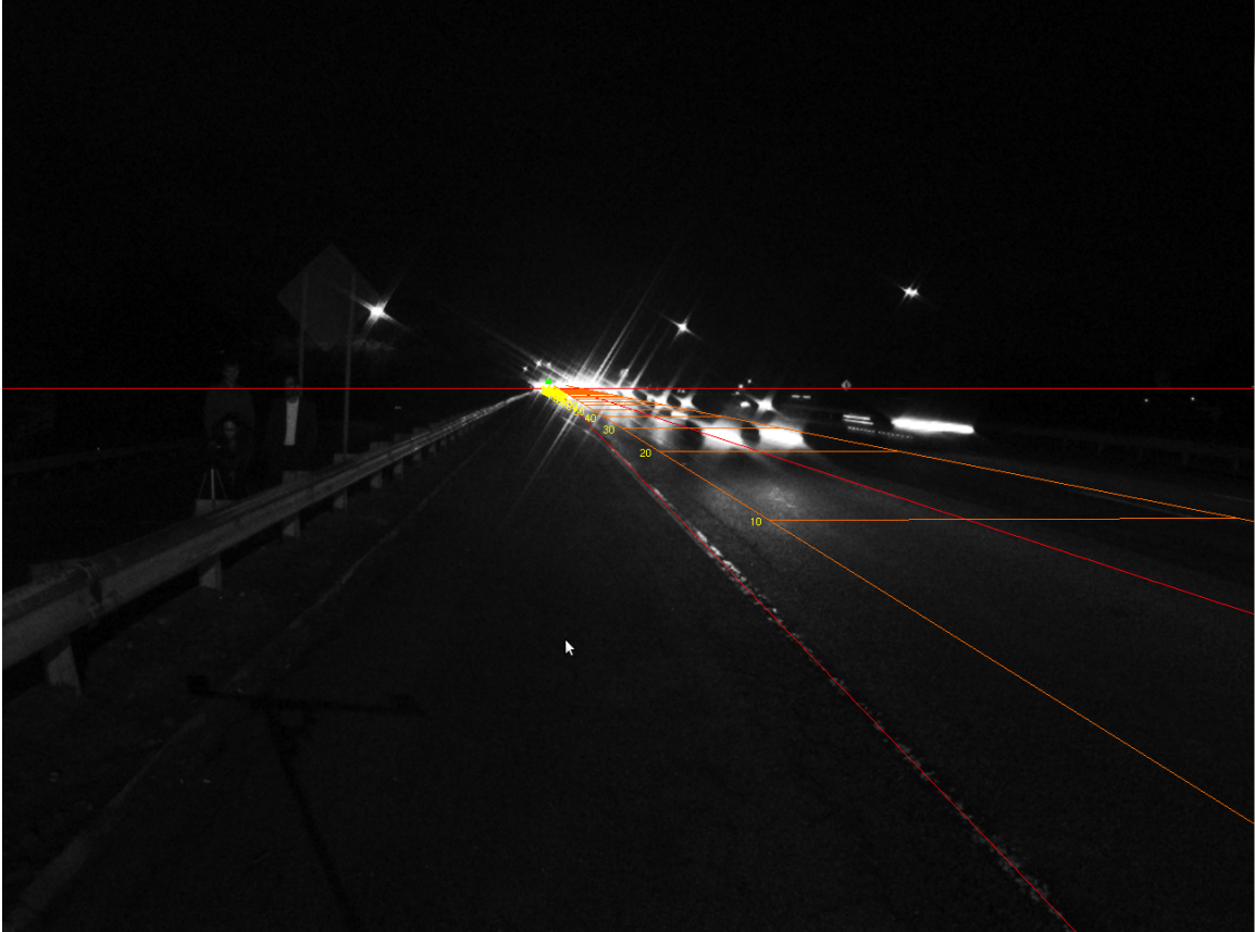
Figure 4-4: The user can toggle the level of the road markings between road level and headlight level. When the road lines are at headlight level, it allows the user to see whether or not the car corresponding to headlights on the screen is within the boundary of the road lane. Notice that the car in the left lane has both headlights between the orange lane lines.
