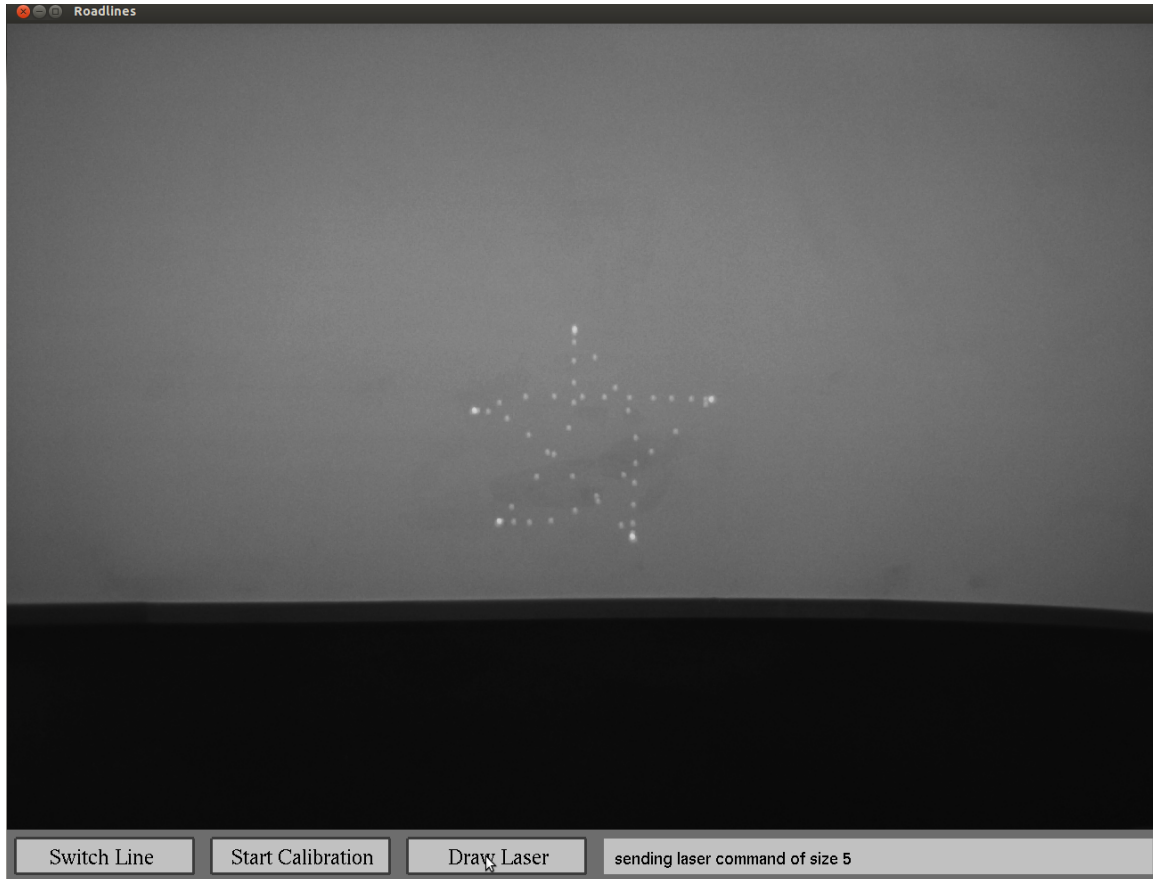
Figure 4-12: Step 5. The user clicks the 'Send Laser' button, and the galvanometer command angles corresponding to the pattern are sent to the laser. Notice the star pattern. The laser in its current state moves between laser points slower than the final laser will, and some intermittent laser points are produced in between each point. Also notice the curve of the lines between each laser point. This is due to the angular nature of the galvanometers, and so the shortest path between two mirror positions does not necessarily translate to the shortest path on the world surface. Finally note that this example of the system uses a flat vertical wall, instead of a horizontal road. This should not make any difference, as the system only assumes a flat surface, and the code has been run on a horizontal surface and works just as well.
