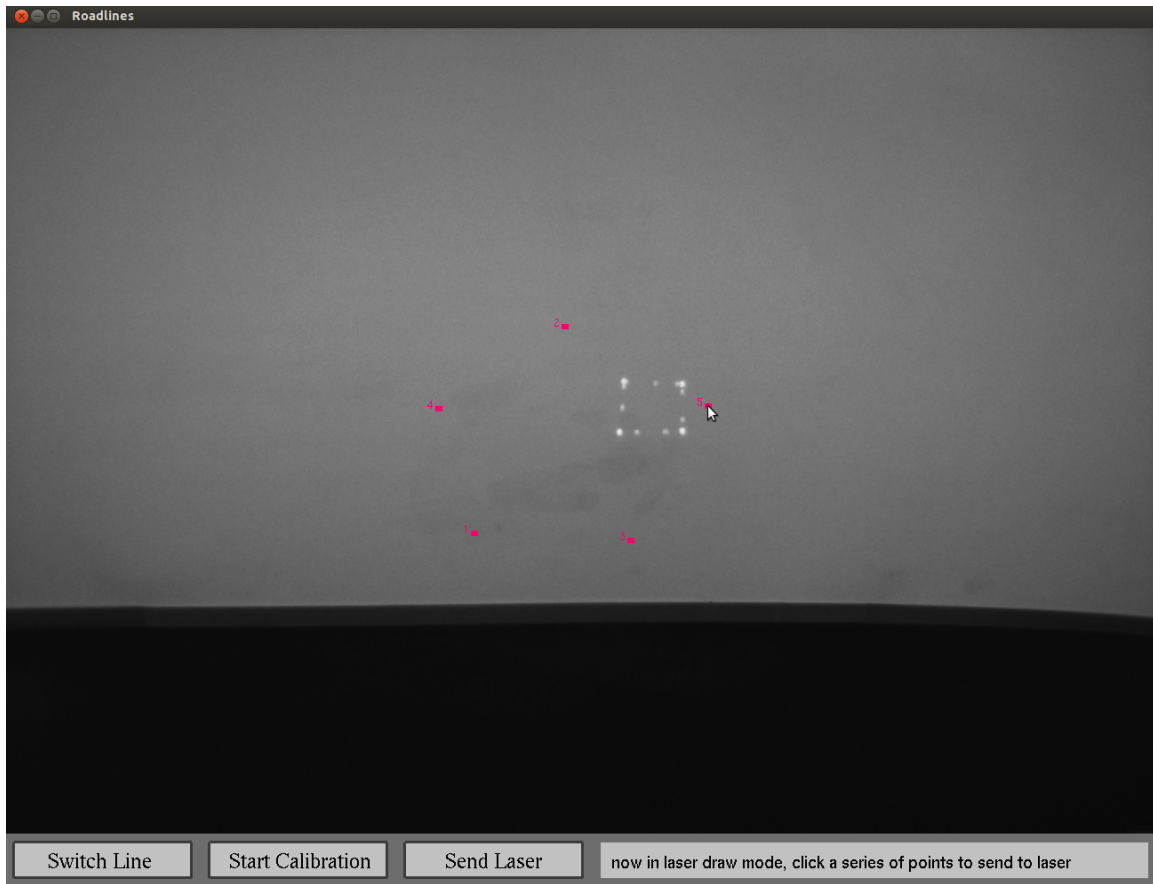
Figure 4-11: Step 4. The user clicks the 'Draw Laser' button, and clicks a series of points in a pattern on the world surface. Notice the order of the points clicked.
