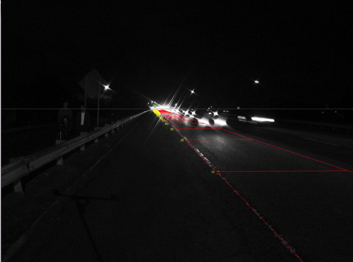
Figure 4-3: The road lines program running on a log of the footage from a ride along with an officer. The user adjusts the road lines shown overlaid on the picture to fit the lines of the road in the picture. The system then automatically calculates the distance to the road, the road width, and a transformation from the camera's coordinate frame to the real world coordinate frame. Based on these calculations, the system then displays meter markings at increments of 10 meters along the road.
