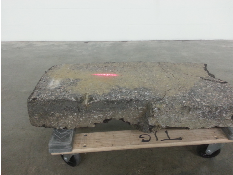
Figure 4-2: Foreshortened PWM Laser spot on Asphalt Sample
