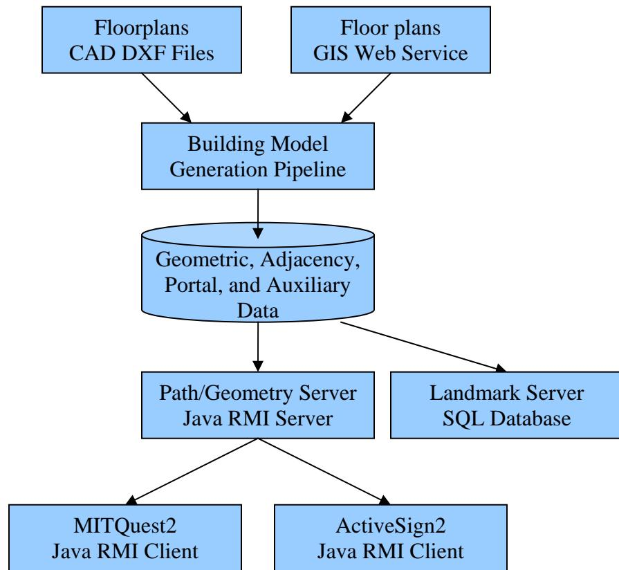
Figure 1: BMG System Architecture
