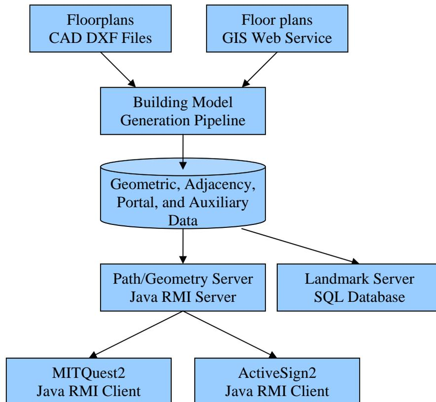
Figure 1: BMG System Architecture
